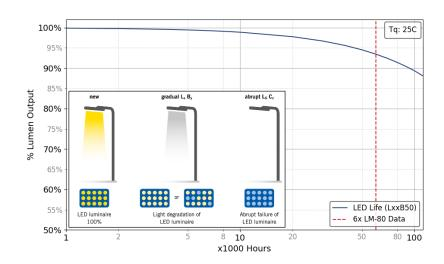
For reference purposes, the graph extrapolates beyond the recommend 6x LM-80 data in TM-21, which our calculations are based on.
